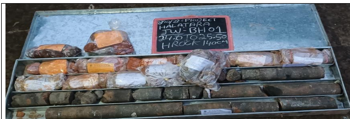
Figure 13: View of the core box of drilling done for Jack well foundation
